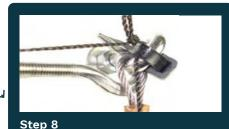
To attach the net to the rope, attach one corner of the net to the corner fixing using a netting corner tie. When you reach each corner ensure that a netting corner tie is installed around the mesh and the corner fixing.
